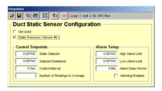
All setpoints related to duct static control pressures and alarm points are programmed on this screen which activates when you left-click on the pressure reading box.
